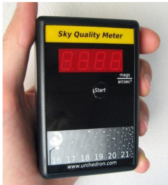
Figure 10 Unihedron Sky Quality Meter - Source: https://commons.wikimedia.org/wiki/File:SQM-L.jpg
